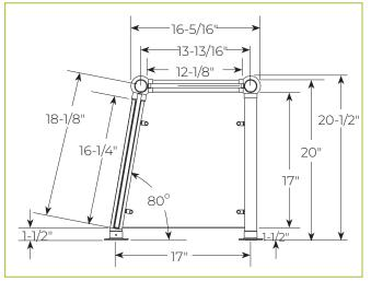
To meet NSF guidelines, end panels are included on all BSI quotations unless specifically excluded. Ships fully assembled.
